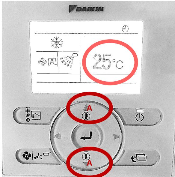
3. PRESS HIGHLIGHTED BUTTONS (A) TO SET THE TEMPERATURE
