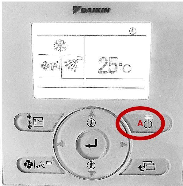
1. PRESS HIGHLIGHTED BUTTON (A) TO TURN ON OR TURN OFF THE DEVICE
