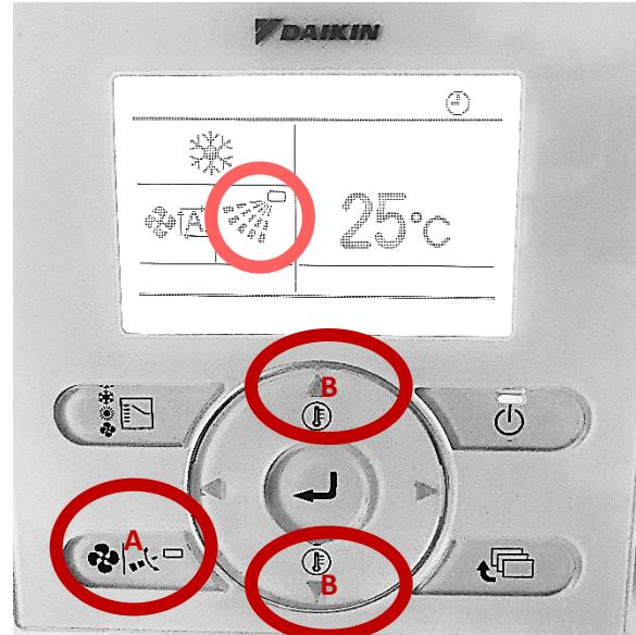
**4. DRÜCKEN SIE MARKIERTE TASTE (A) UM DIE WINDKRAFT ZU WÄHLEN**
