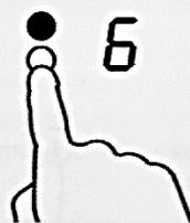
2. Turn the cooking zone off by scrolling down to "0" or touching "-" and "+" control together.
